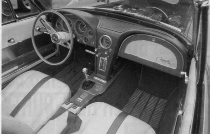
The interior of the Knudsen car (above) is anything but stock. Note the floor grilles, steering wheel and door panels. Seats are genuine leather. Enginewise (below), a stock but prettied-up fuelie powered the car. The battery had to be relocated to the trunk to make room for the exhaust headers.
